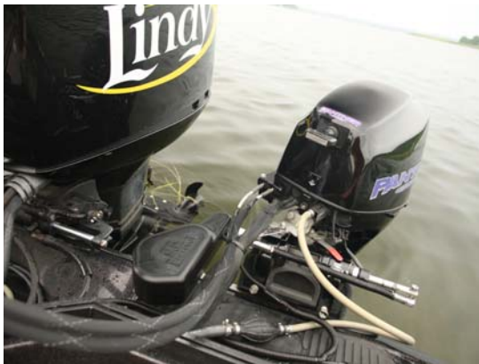
Installed T-5 on kicker engine
