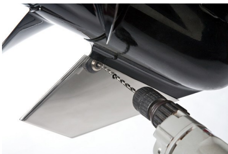
Drill two holes
