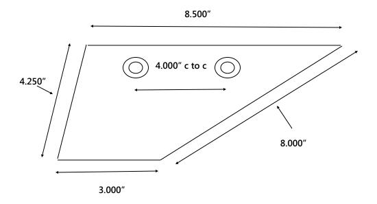
Made of 316 Marine Grade SS 1.5mm material thickness
