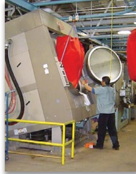
450# two way tilt washer extractors are easily sling loaded.
