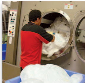
Milnor large open pocket washers can be sling loaded.
