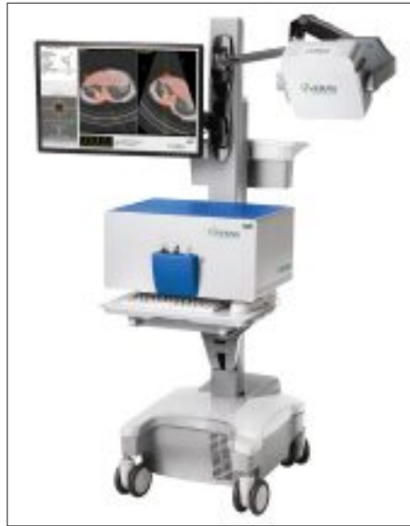
Veran's ig4 platform uses electromagnetic-based, 4-D navigation technology for interventional radiology.
