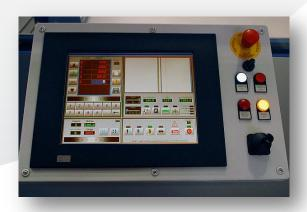
On large conveyor systems a PLC with Touch Screen can be easier to operate and more cost effective than manual buttons and switches.
