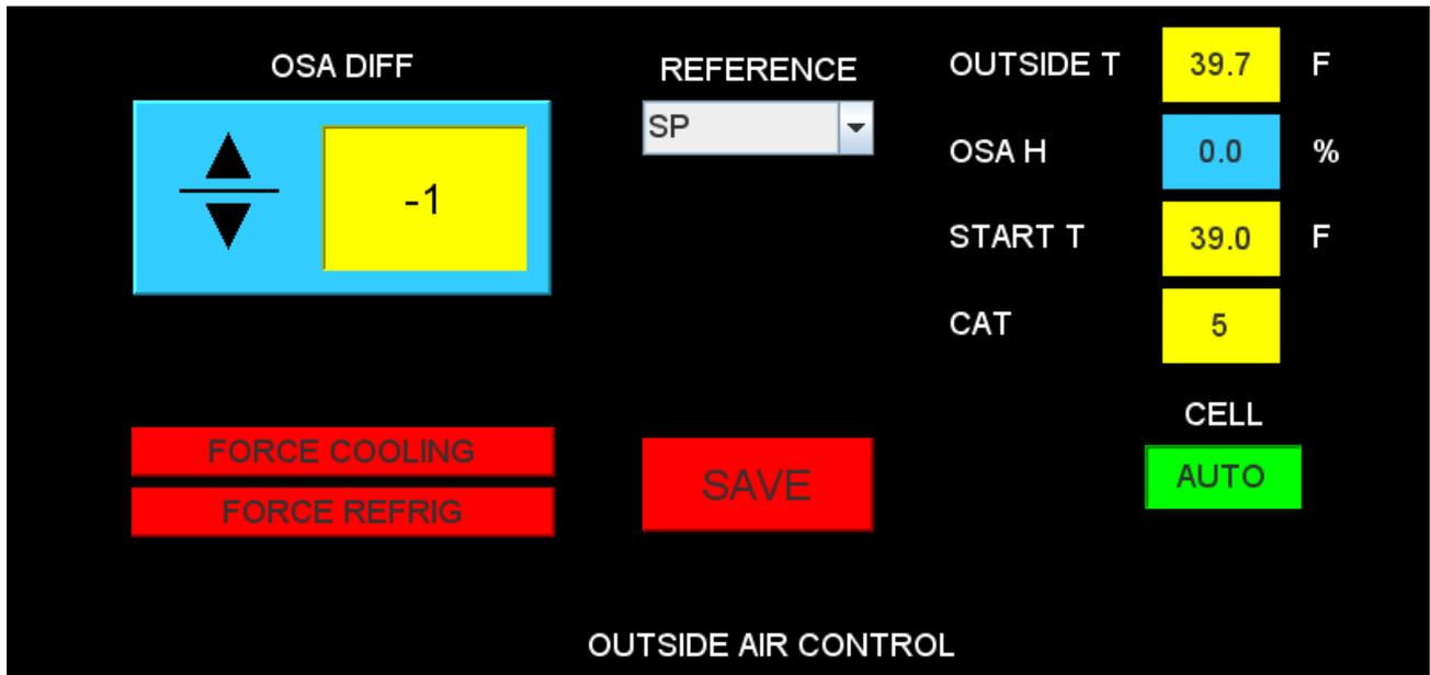
The OUTSIDE AIR CONTROL screen allows for the setting of the outside air differential and the reference. These values are used to calculate the START T. Any time the Outside air temp is less than the Start temp
