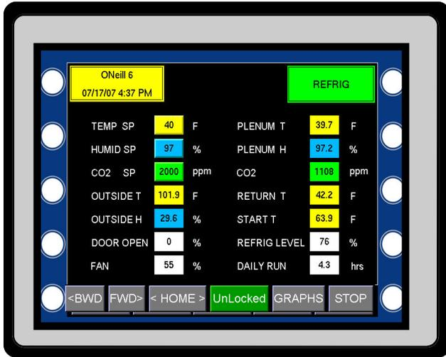
Pressing the GRAPH button from any screen will access the Graphing module
