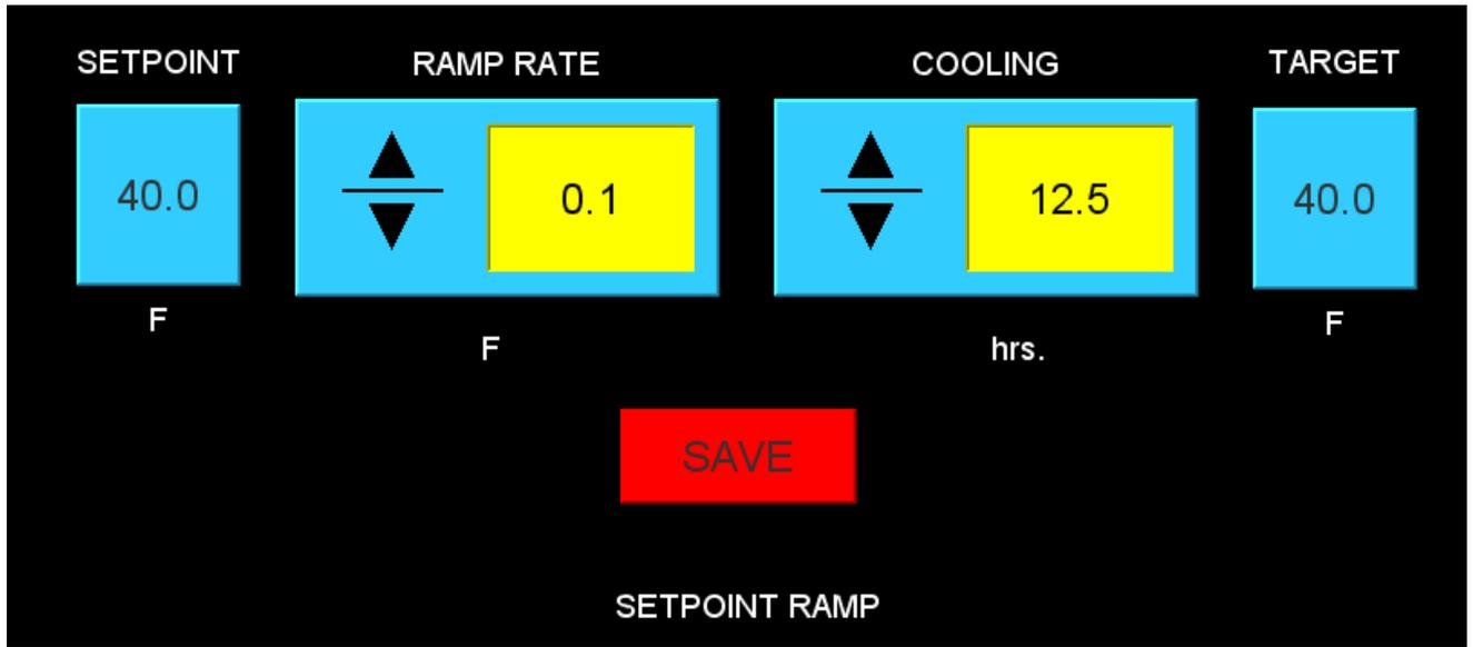
The Setpoint Ramp screen allows the ramp to be set up just like the HMI screen.
