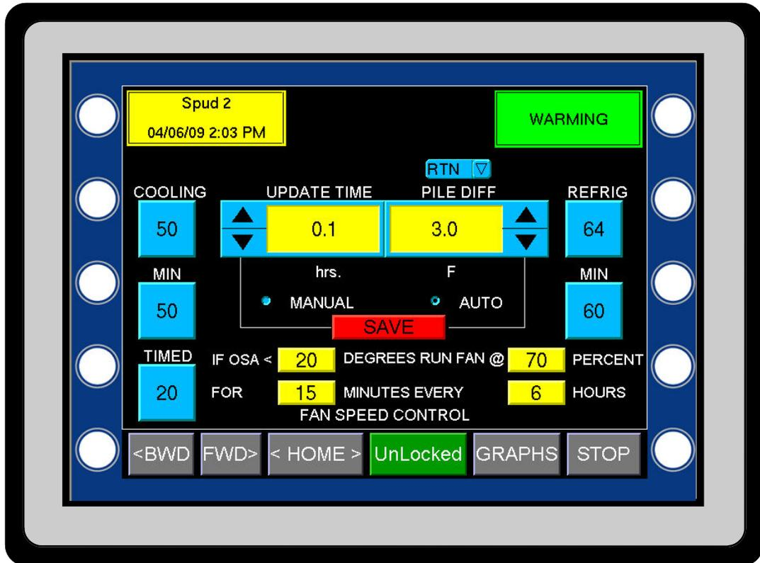
The FAN SPEED CONTROL screen allows the user to set up a number of parameters that will control the speed of the fans. Each of the five button can be programmed by pressing the button and then entering the value.
