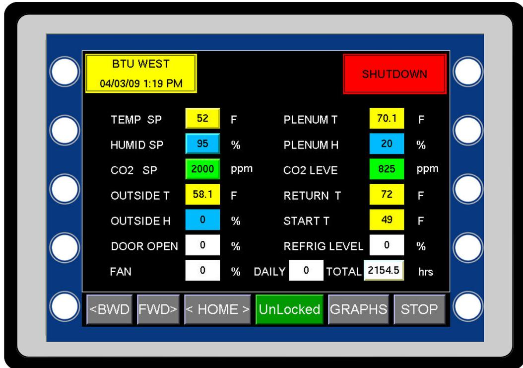
**2.1 G70 HMI (Human Machine Interface) color touch screen:** The XT panel has many options for user interfaces. The standard interface is a G70 and is a 320 x 240 color touch screen. An optional G75, 640 x 480 larger color touch screen, is also available. Active touch buttons are either labeled or shown as raised buttons. Pressing one of these buttons will produce a keypad for entering a new value.
