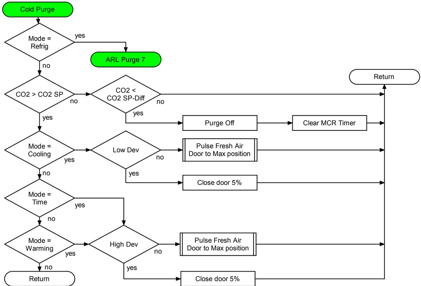
If the system is running in Cooling and the CO2 level exceeds the CO2 Setpoint, the fresh air doors will be pulsed open to the Max door setting. If during this opening of the fresh air doors, the plenum temperature drops below the Low Dev setting, the doors will be closed 5% until the plenum rises.
