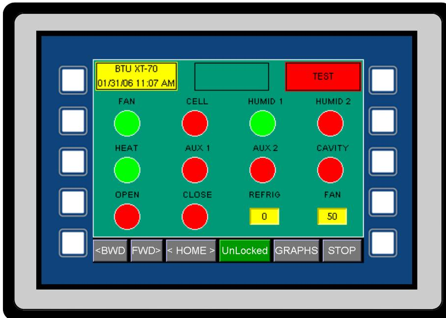
When the XT panels goes to the Test mode, all normal operation is suspended.
