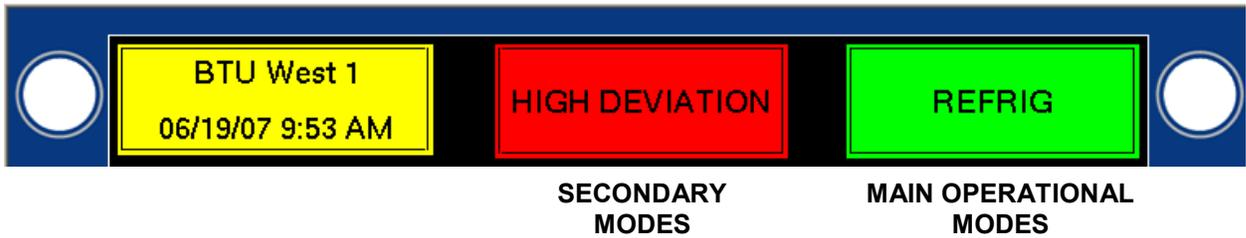
**XT Modes:** The XT Panel operates in two modes: the main operation mode and a secondary mode. Depending on the setup of the alarms, it is possible to continue running in an alarm mode.
