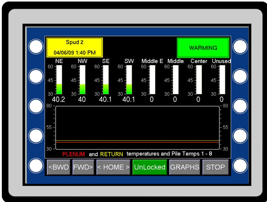
Each of the pile temperatures are displayed as a bar graph and in a window. The bar graph allows easy comparison between all of the pile temperatures. If the system is operating a cavity, some of the pile sensors may be designated as cavity sensors.
