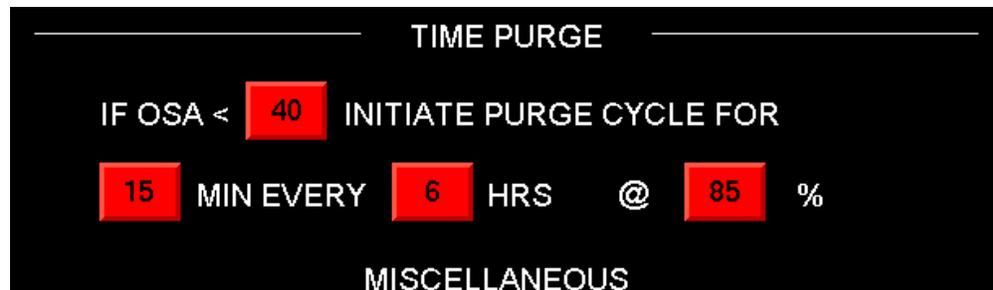
Four parameters must be set to initiate the time purge. In the above example if the outside air is less than 40 degrees initiate a purge cycle for 15 minutes every 6 hours and set the fans
