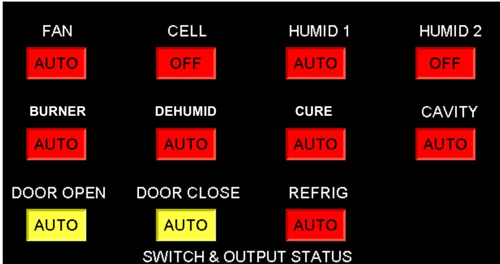
This shows the HMI layout, the actual switches on the panel need to be relabeled.
