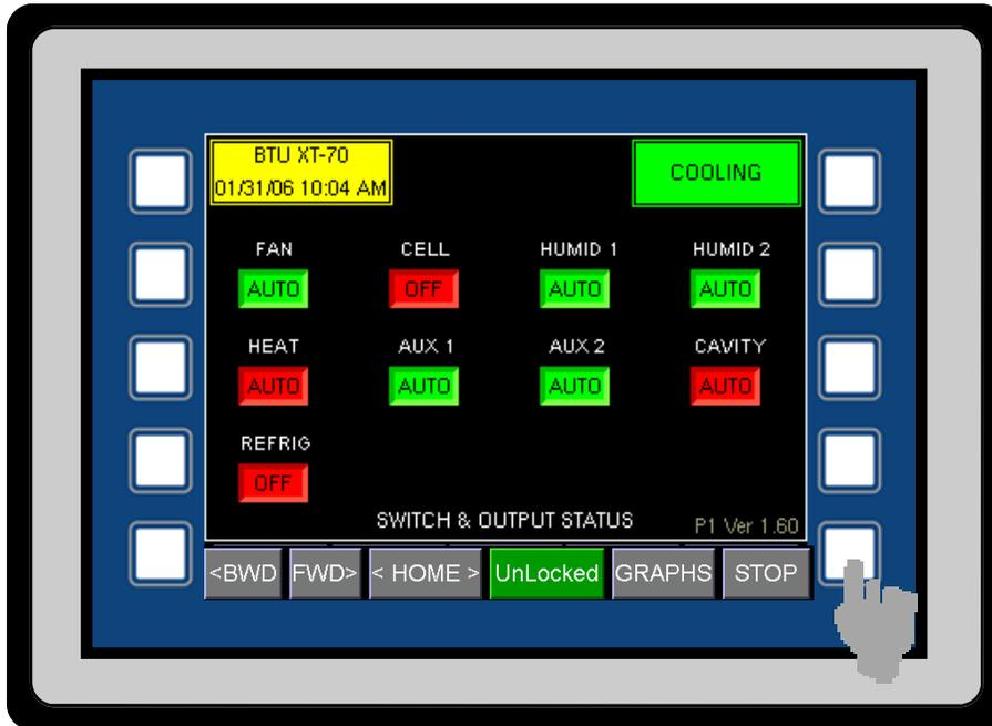
In order to place the XT panel into a test mode, first go to the SWITCH & OUTPUT STATUS screen. Once at this screen, press the bottom right outside button.
