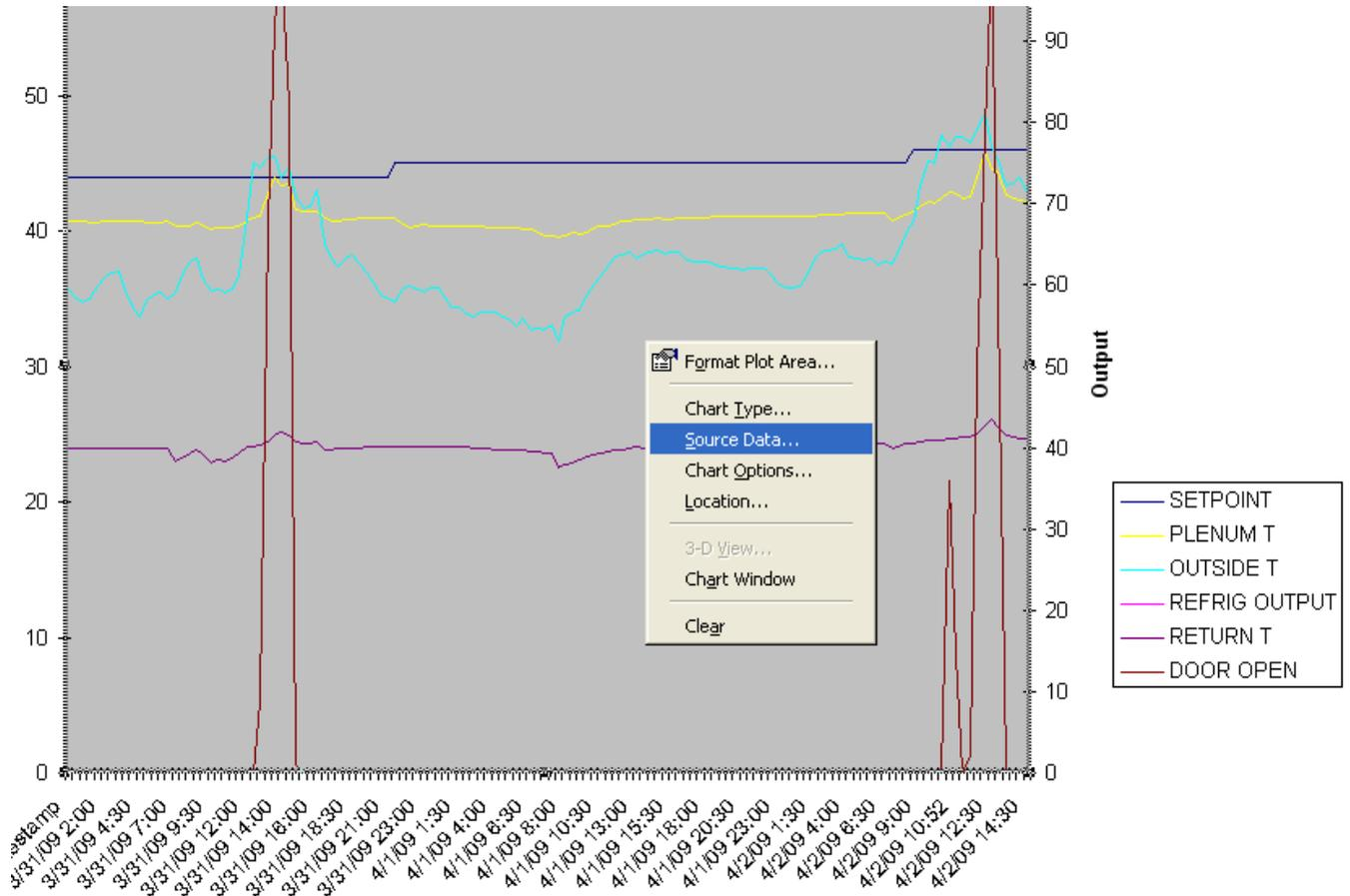
To make a change to the parameters being graphed, right click on the graph and select Source Data. Remove parameters by clicking on the parameter and then Remove. To change a parameter, select the parameter, determine which column the needed parameter is in and then change the alpha character in both the Name and Values boxes.
