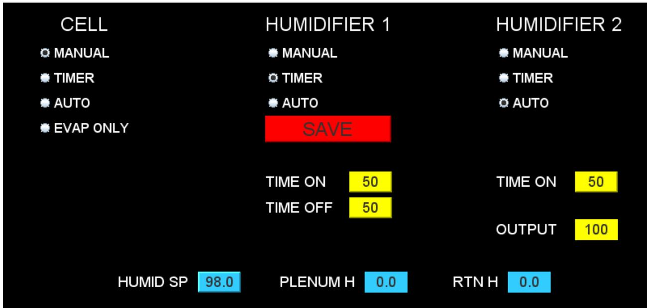
The Humidity screen allows all the humidity parameters to be set. See section 5.10 for more information.
