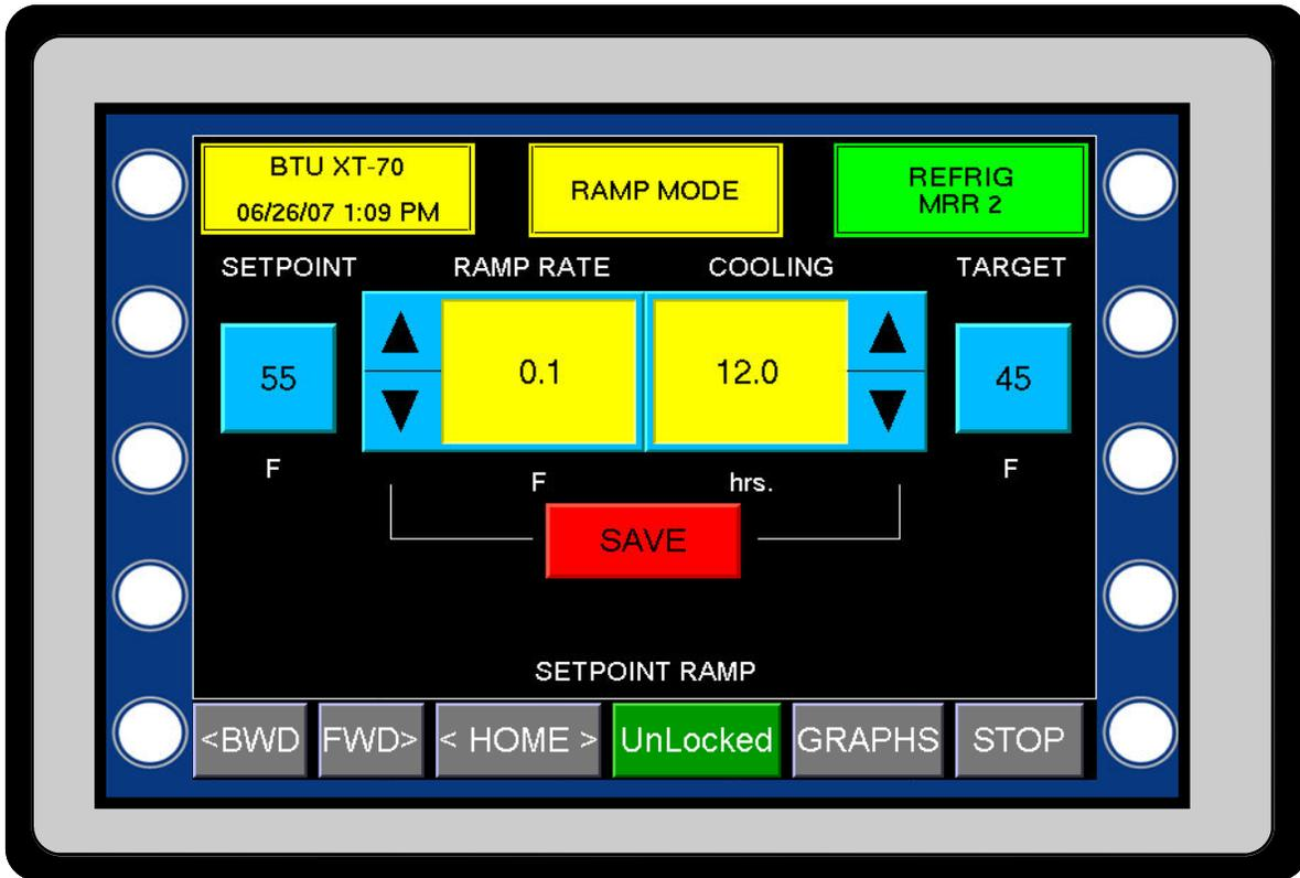
The SETPOINT RAMP screen allows the user to set up the ramp function. The ramp function will allow the setpoint to be automatically incremented to a target setpoint. An example of this could be seen in the fall. Once suberization has taken place, the ramp function could automatically drop the setpoint in small increments until the target temperature is reached.
