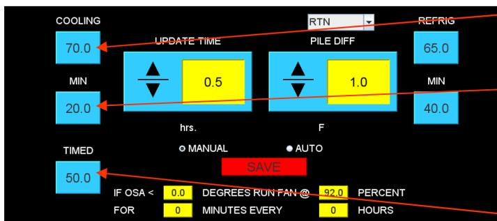
The Cooling button is the Max fan speed. The door position can go to 100%, but the fan will go no higher than this percentage. The MIN button on the left controls the minimum speed of the fan when the Door Open is zero. For example, if this is set at 20%, the exhaust fan can not slow down to less than 20%.
