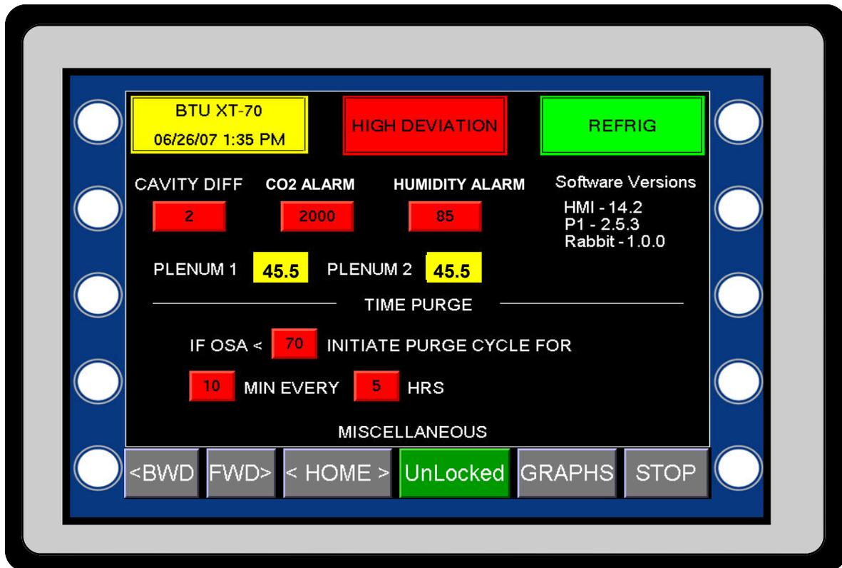
CAVITY DIFF: the cavity differential is a +/- variable and is programmable by pressing the button. The cavity differential will help determine when the cavity heat will turn on and turn off. Typically, the pile 2 sensor is the controlling sensor and is located on top of the pile. Pile 8 would normally be the controlling cavity sensor. The XT panel allows setup for different controlling sensors. The example below explains how the cavity works.
