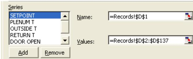
To add a button, click on Add. Then go to one of the other sensors and copy the Name string and paste it in to the new one and change the alpha character to match the desired value. Repeat for
