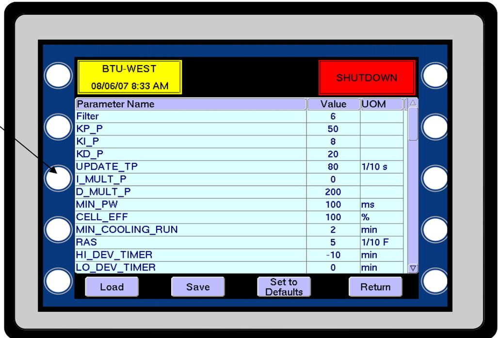
To change a parameter, press the value and a pop-up keypad will appear. Enter the desired number. Make multiple changes, if desired, and ,when done, press Save and then Return. If Set to Defaults is pressed, the default values for all parameters will appear. They are not saved until Save is pressed. Pressing the Load button will load the screen with the current values.
