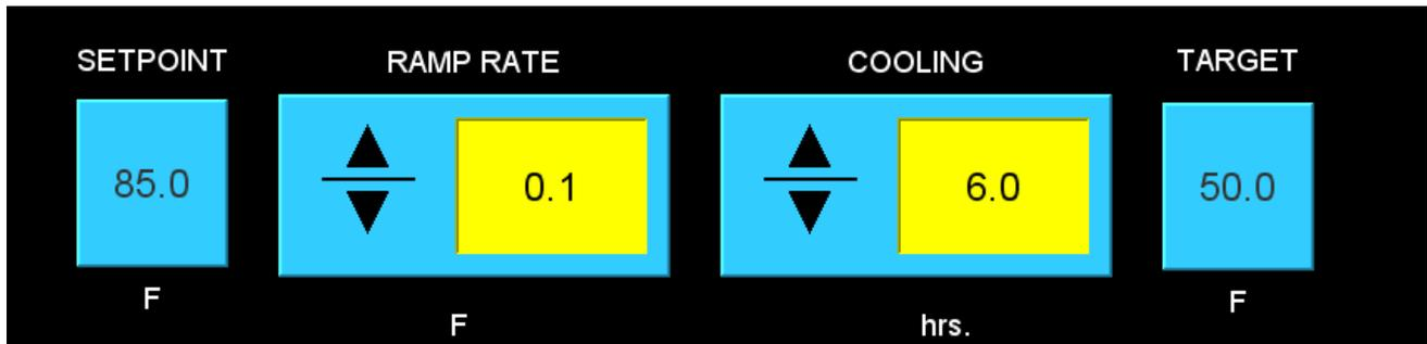
In this example, the Setpoint will be ramped down .1 degrees every 6 hours of Cooling. The ramp will shut off when the final Target temperature of 50 degrees is reached. **Note - anytime the Setpoint is changed from the main screen, the Target will be reset to the Setpoint and the ramp will be turned off.**
