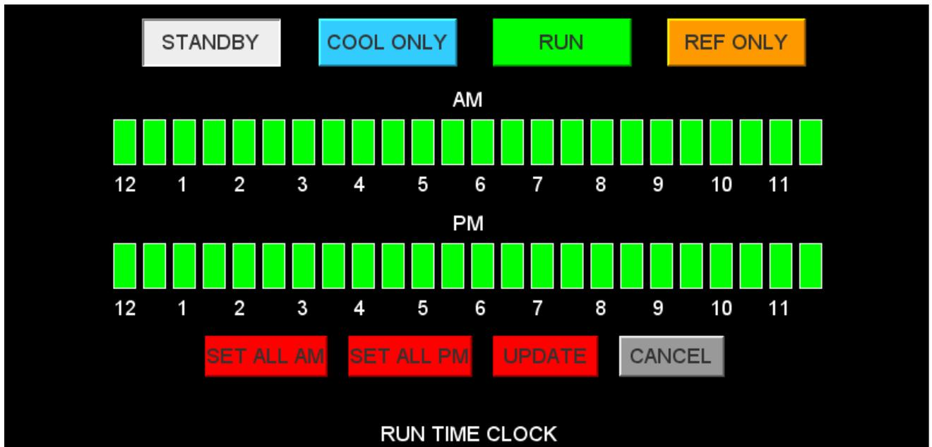
This screen shows the run time clock. To change click on the desired mode, STANDBY, COOL ONLY, RUN AND REF ONLY then click on the desired times. To save click on UPDATE. The SET ALL AM and SET ALL PM buttons can be used to set all the clock increments.
