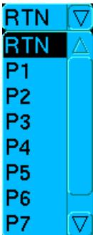
It is highly recommended that the RTN sensor is always used for the pile differential, but under certain conditions, it may be desirable to use one of the pile sensors. The drop down box is used to choose one of the pile sensors.
