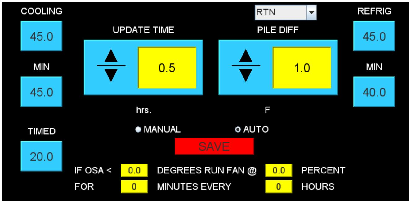
The Fan Speed Control page allows all setting for the speed of the Fan. See section 5.9 for more information.
