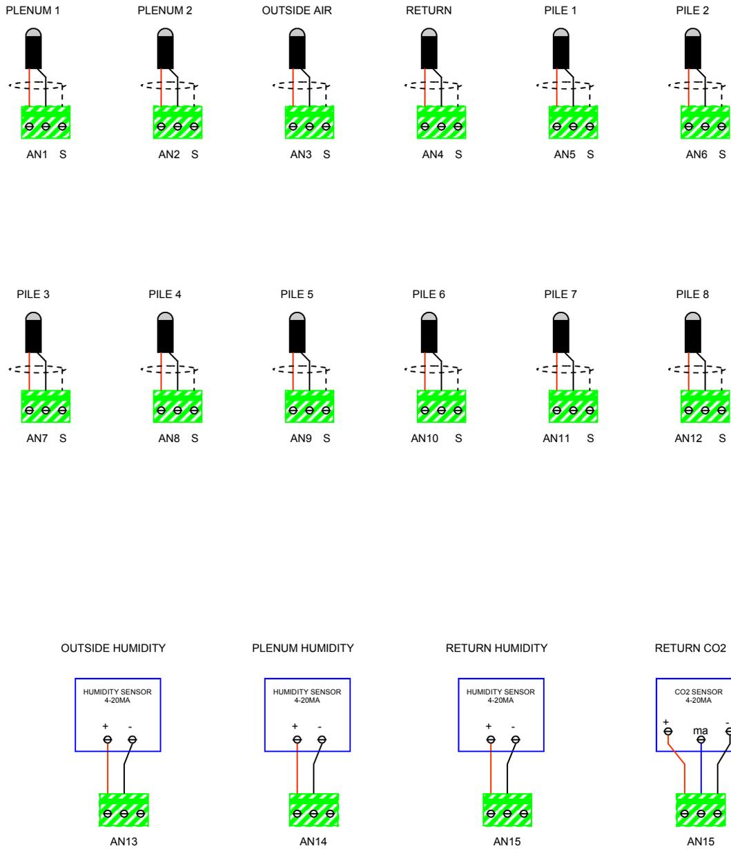
LOW VOLTAGE SENSOR FIELD WIRING
