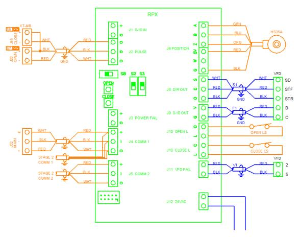
This diagram is for a single stage. The stage has a pulse sensor that keeps track of the exact door position. The board receives open and close pulses from the XT panel on J2. J4 & J5 is used for communications. Forward and Reverse inputs to the drive determine the direction. A 0-10vdc analog output determines the speed and a VFD fault contact is supplied to the card.
